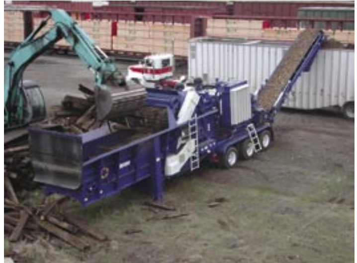
The adjustable Peterson Impact Release System releases to allow uncrushable items to escape from the grinding chamber
